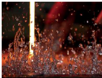
Frit is melted at 1450 °C
