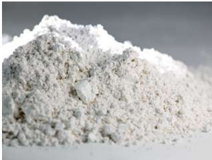
Zirconium silicate gives glaze its white colour
