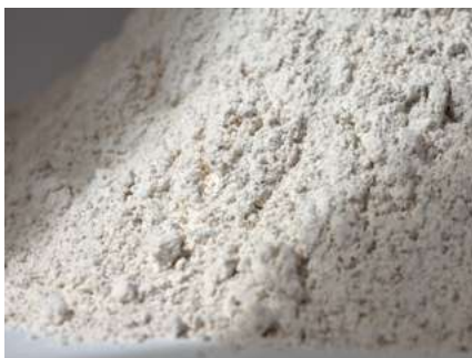
Feldspar, the main component or frit production
